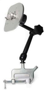
Allows you to fix any types of sensors (resistive or optical) on any circuit breakers.
