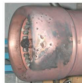
Arc pitting on fixed contacts
