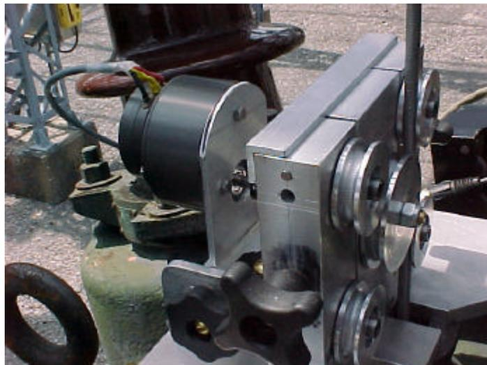
With a **our KIT-ZLR** linear-to-rotary motion converter and a **ZRT-05** rotary transducer.
