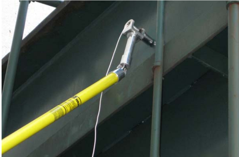
Figure 2 : Pole designed for installation of the accelerometer in height.
