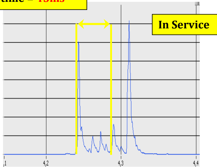
Figure 11 : ABB UCLRN switching at tap -4 in mode In Service
