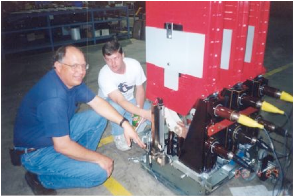
Linear displacement mechanism mounted on a small air breaker.
