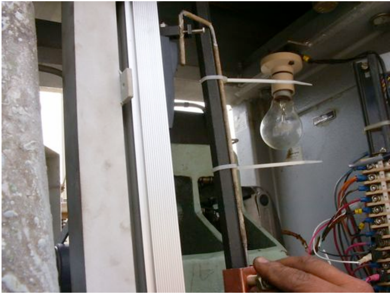
Steel rod attaching the base and the linear transducer to the mechanism.
