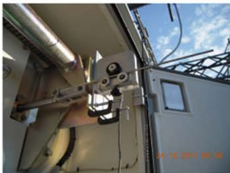
With a resistive displacement transducer Ref : ZRT-01/03/05/10
