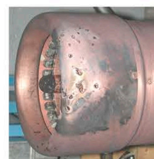
Arc pitting on fixed contacts
