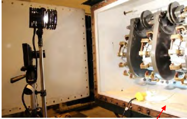
Fig. 1.5 Connection of contact clamps on the transformer
