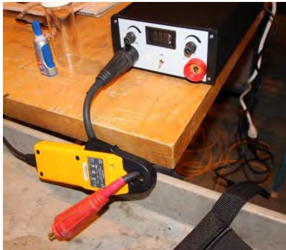
Fig. 1.4 DC voltage source and current clamp
