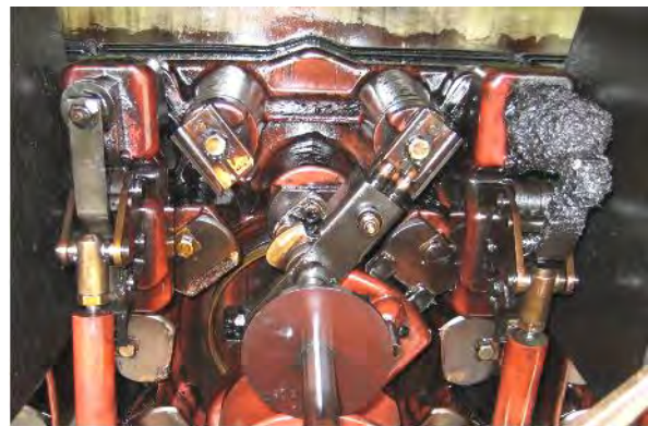
Fig. 1.14 Coking and burnt contacts of a TC-546
