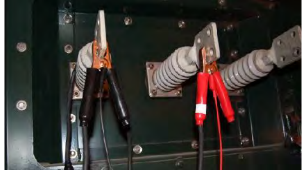
Fig. 1.5 Connection of contact clamps on the transformer
