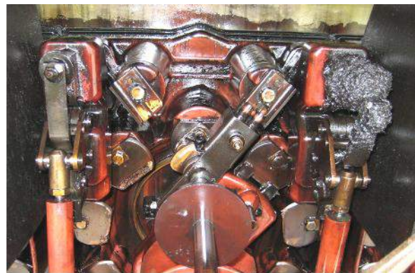
Fig. 1.14 Coking and burnt contacts of a TC-546
