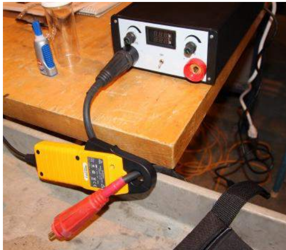
Fig. 1.4 DC voltage source and current clamp
