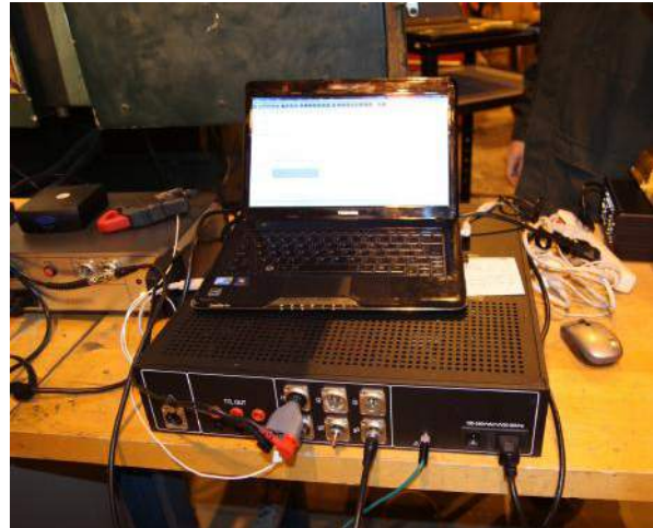
Fig. 1.1 Zensol OTM-X - Instrument for the acquisition of vibration, current and voltage signals.
