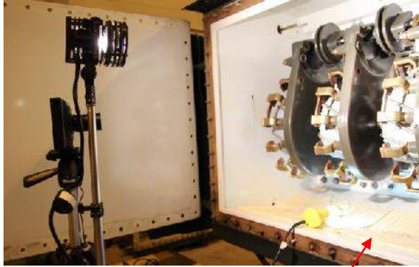
Fig. 1.5 Connection of contact clamps on the transformer
