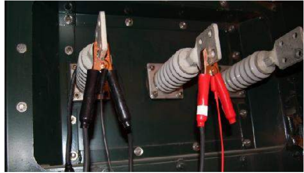
Fig. 1.5 Connection of contact clamps on the transformer
