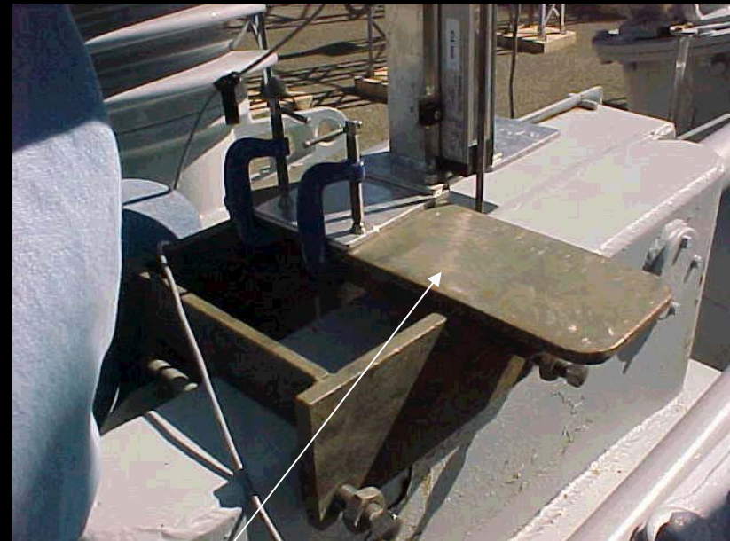
Mechanical basis allowing the positioning of the transducer on the breaker
