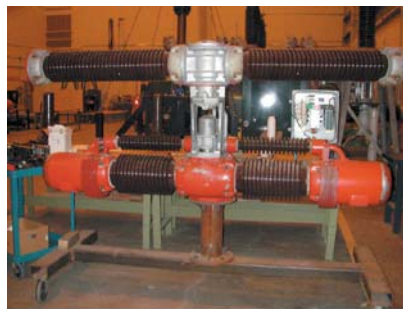
Fig 9 DLF air-blast breaker module
