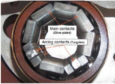
Fig 7 Tulip contact in oil circuit breaker
